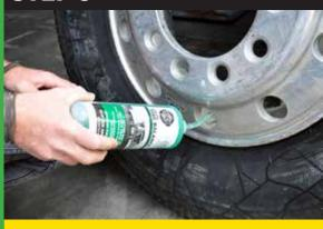
Connect Hose to Valve Stem and Squeeze Bottle to Fill.
