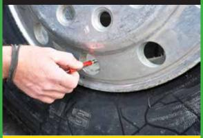
Remove Valve Core to Release Air From Tire Completely.
