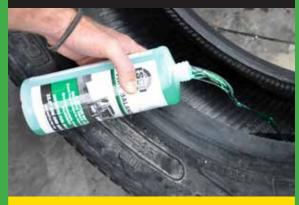
Liquid Tire Balance Can Also Be Installed
